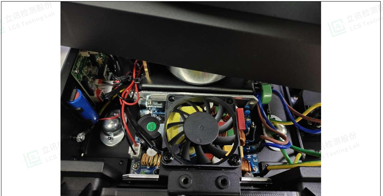
Photo 26 LED driver for front end
