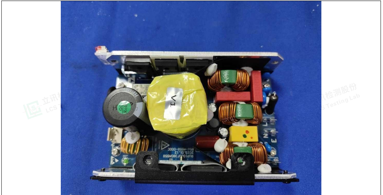
Photo 27 LED driver for front end
